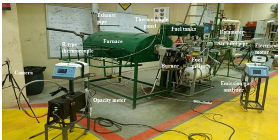
Figure 2. Direct photo of the testing apparatus in the laboratory
