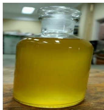
Figure 4. The sample of mixture biofuels D50B50E15 At the National Research Centre (NRC-Dokki), Egypt, the properties of diesel, D50B50, and bioethanol characteristics of the tested fuels were measured by ASTM standards as given in Table 3
