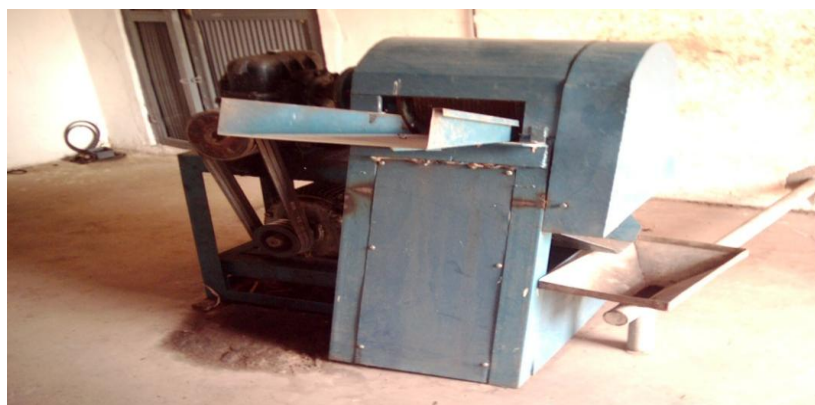
Fig 1: Cane Crusher Designed and Fabricated by NCRI for the production brown sugar.
