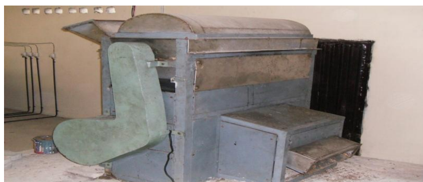
Fig 2: Cane Cutter designed and fabricated by NCRI for the production of brown sugar.
