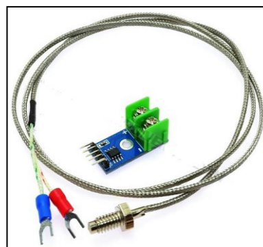
FIGURE (4):MAX6675 K-TYPE THERMOCOUPLE
